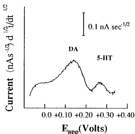
FIG. 1. A semiderivative voltammogram showing the in vivo electrochemical detection of DA and 5-HT in freely moving and behaving male Sprague-Dawley rats. Peak potentials for DA and 5-HT were  $0.140 \pm 0.015$  V and  $0.290 \pm 0.015$  V, respectively. Dopamine and 5-HT release were detected with a temporal resolution of 10-15 s and 10-12 s, respectively.
